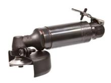
All steel housing with push back safety lever throttle. Used for grinding, deburring and blending. Features a wick lubrication system and spiral bevel gears. Equipped with 4" guard, dead handle and adjustable side exhaust.
